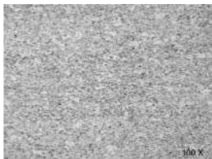
Figure 12 In-situ metallography of Water Tube Compartment 2 (West), Tube No. 2 Layer 1 (Material: BS 3059 Part 1:1987 Gr.320 ERW). (A) Microstructure at 100X magnification indicating a normal condition with a ferritic matrix (white) and sulfide impurities (black)
