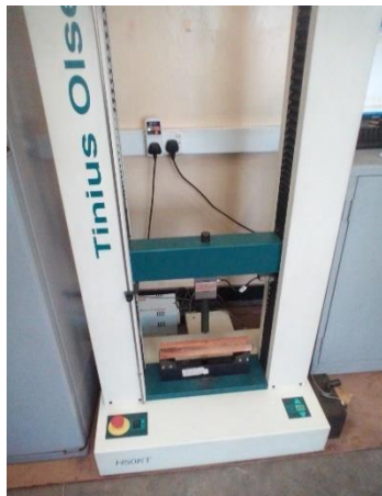
Figure 4: Test process for the flexural properties of Eucalyptus glulam
