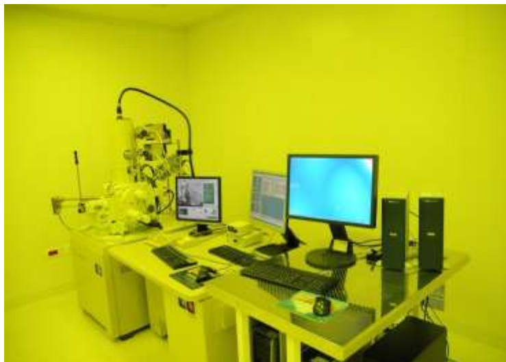
Figure 6: Scanning Electron Microscope, photo taken from BioNano Technology Research and Development Center, Fatih University, Istanbul, Turkey.
