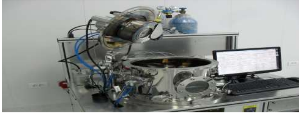
Figure 2: RF and DC Magnetron Sputtering Deposition, photo taken from BioNano Technology Research and Development Center, Fatih University, Istanbul, Turkey.
